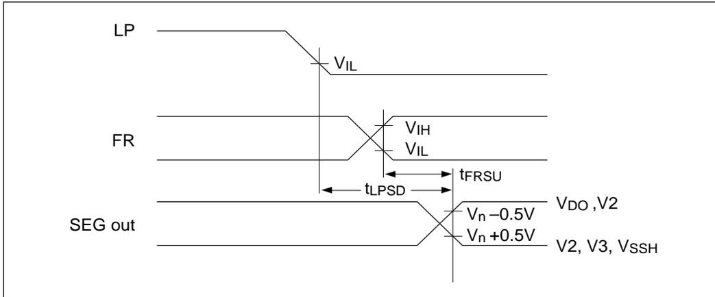
$V_{IH} = 0.2V_{SS}$ ;  $V_{IL} = 0.8V_{SS}$  ( $V_{DD} = 0V$ ,  $V_{SS} = -5.0V \pm 10\%$ ,  $T_a = -20$  to  $75^\circ C$ )
